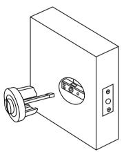
7 Insert the release, with the rapidFIT and spindle attached, into the 48mm hole and press against the door.
