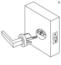
6 Insert handle 'A' in the 48mm hole with the spindle and rapidFIT attached and press against the door. Ensure the grooved side of the spindle is aligned with the grubscrews on the handle
