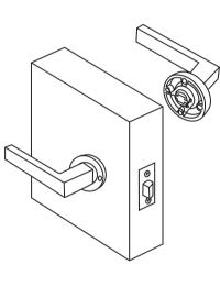
**Note:** The grubscrews may need a re-tighten after a bedding period. We recommend medium strength thread-lock to bed used.
