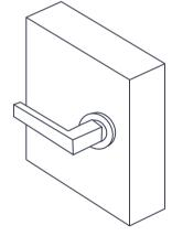
6 Screw the rose cover onto the handle and tighten the grubscrew on the side of the lever onto the spindle.
