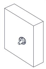
3 Fill the dummy spindle by drilling and fitting the three wood screws provided. Ensure the grooved side of the spindle is aligned with the grubscrews on the handle.
